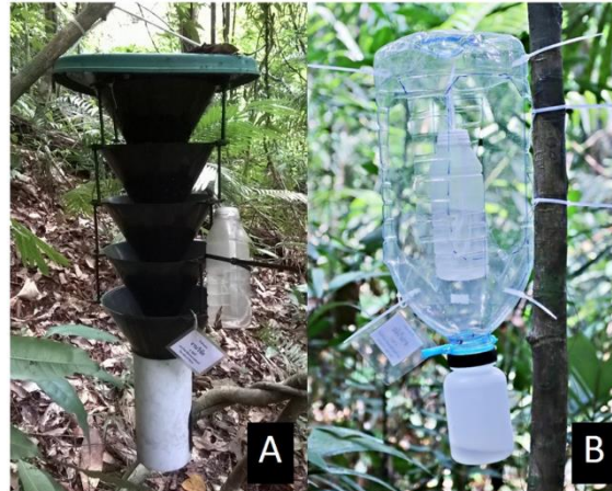
Figure 2 Trap types using in the experiment A) Lindgren-5-funnel trap B) 5-liter Bottle trap
