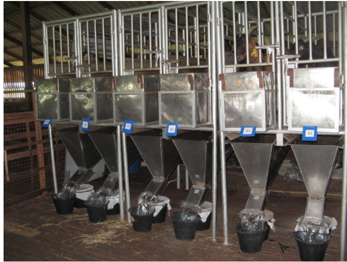
(m) Metabolism crates, goats and equipment for total collection of feces and urine
