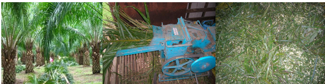
(h) Oil palm leaflets, chopping and oil palm front after chopped into lengths of about 2 cm
